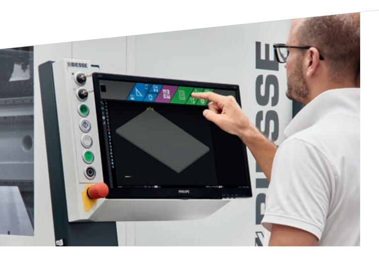
bTouch is the new 21.5" touch screen which enables you to carry out all of the functions previously performed using the mouse and the keyboard, enhancing the direct interaction between the user and the device.
