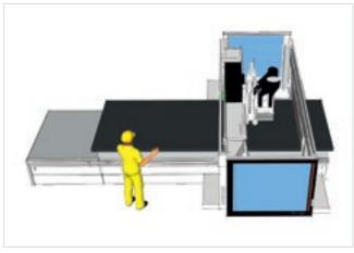
The machine can be configured with tandem loading in order to alternately process panels on opposite origins. This allows loading and unloading to be carried out while the machine is actually running.
