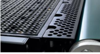
Chip removal system positioned between the machine and the unloading belt, guaranteeing optimal panel cleanliness.
