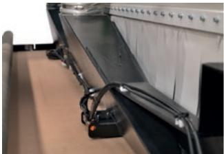
**Sweeping arm** with adjustable blade and copying system. The device allows the automatic offloading of panels up to 3mm thickness.
