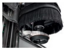
The **loop presser** supports the machining of warped and overlapping panels of breathable material, or those with a high level of friction, by applying pressure to the upper surface of the panel.
