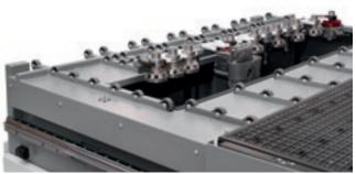
The magazine is integrated into the base, ensuring that tools are always available even when using automatic loading solutions whilst keeping overall dimensions to a minimum.
