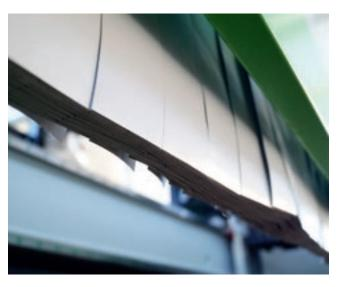
Overlapping lateral curtain guards protect the working unit.
