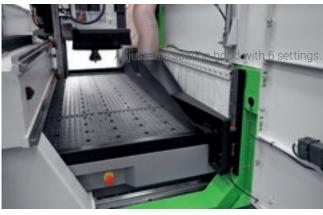
The **sweeping arm** with integrated suction supports the simultaneous cleaning and unloading of panels, avoiding manual intervention and thus increasing productivity.
