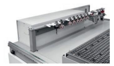
Tool change magazine with up to 14 spaces, rendering all tools and aggregates available at all times with no need for operator intervention when changing tooling between machining operations.
