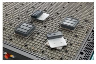
Work table in phenolic laminate with vacuum system.
