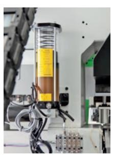
Automatic lubrication is an option that ensures the continuous lubrication of the machine's main moving parts without the need for operator intervention.
